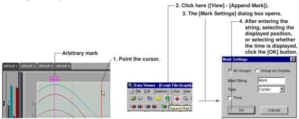
When Cursor A and Cursor B are at the same position, arbitrary marks can be placed. You can select whether to put the arbitrary marks on all groups or only on the displayed group. And you can set the displayed position of the mark and select whether the time is displayed by the mark. The displayed time is either the absolute time or relative time depending on the time axis setting.
