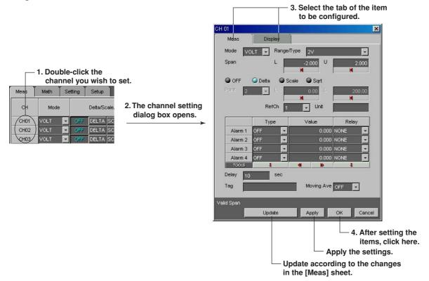
The items in the measurement channel tab can be configured for each channel. The items that are configured are the same as those configured on the spreadsheet. For details, see the page corresponding to the item.
