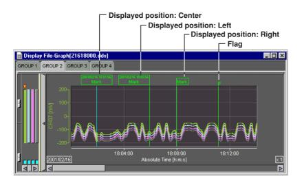
If you left-click the mark while pressing the "Ctrl" key, the mark is displayed in front. If you left-click the mark while pressing the "Shift" key, the mark is displayed in the back. Double-clicking a mark, that has been created using the Data Viewer, opens the [Mark] dialog box in which you can change the displayed group and the mark name.
