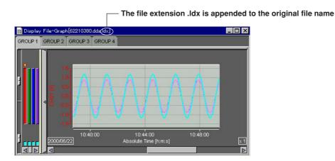
When linking and displaying files, make sure that the number of data points after linking does not exceed 1048576.
